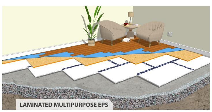
Amdry Eco is a non-structural rigid insulation panel made from closed cell, molded Expanded Polystyrene (EPS) with a layer of High Impact Polystyrene (HIPS) film. The laminated side has bi-directional  $\frac{1}{2}$ " (13mm) wide by  $\frac{1}{2}$ " (13mm) high channels that can be used for venting or water drainage, depending on the application.
