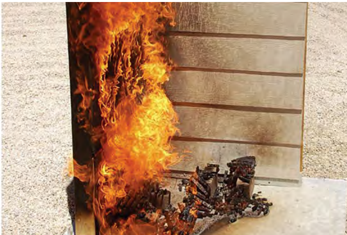
Siding Test. A burning brand applied to a test wall assembly at UC Davis set alight the composite wood siding (left side), but the fiber-cement-covered wall did not ignite.
