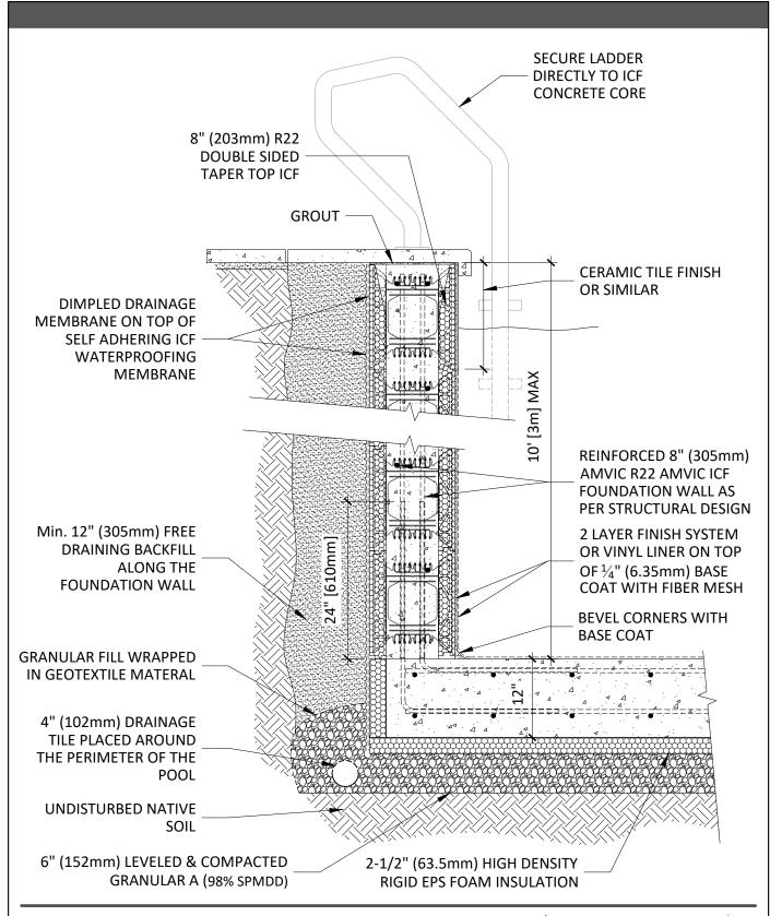
8" R22 AMVIC™ ICF POOL FOUNDATION WALL W/ 12" CONCRETE SLAB
