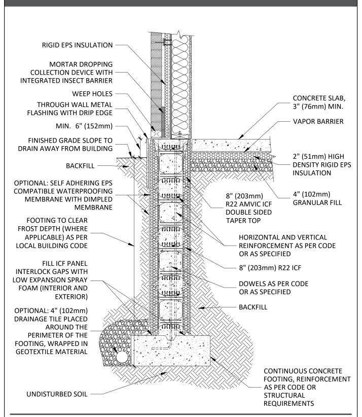
8" R22 AMVIC™ ICF FROST WALL TO WOOD FRAME WITH SLAB ON GRADE
