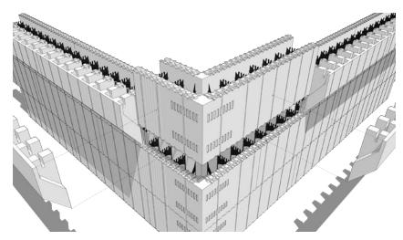
Figure 31 – Regular corner blocks can be used at the same course as the brick ledge forms
