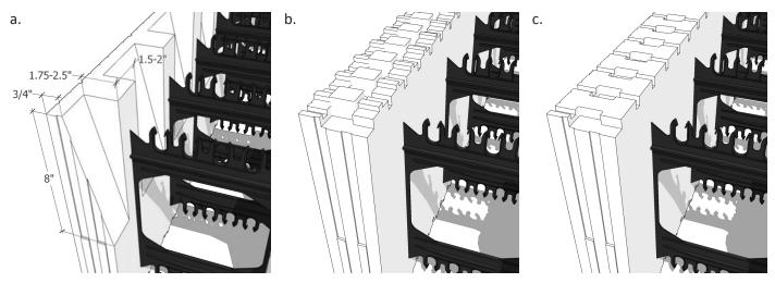
Figure 54 – Typical taper top block (a), typical straight block (b), straight block after interlock removal (c)
