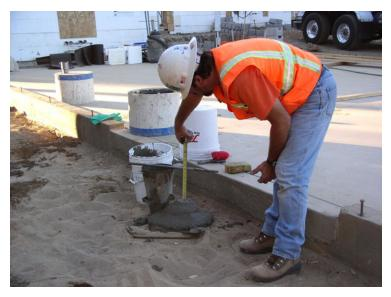
Figure 11 – Performing the slump test in the field
