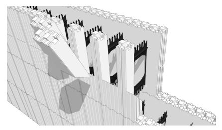
Figure 28 – Cut the EPS foam between the webs as per spacing on the drawings
