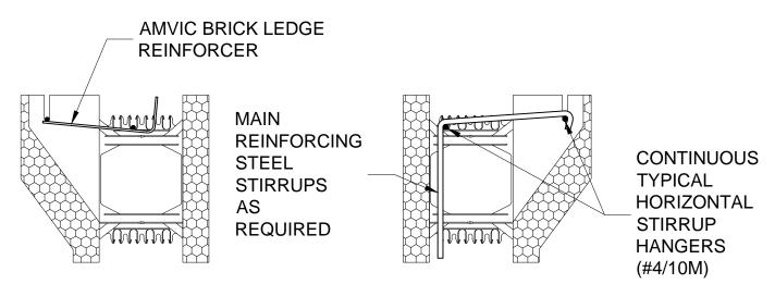
Figure 21 – Cross section of 8" (203mm) brick ledge form with the Brick Ledge Reinforcer or conventional stirrups
