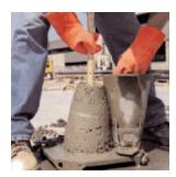
Figure 4 – Concrete mix with low slump
