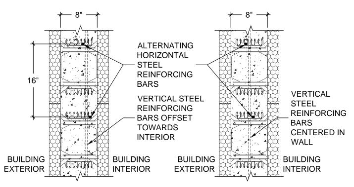
Figure 1 – Typical reinforcing steel placement below (left) and above (right) grade
