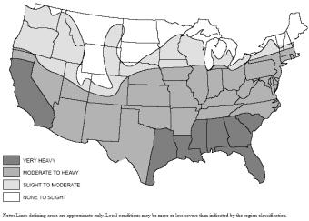
Figure 8 – Illustration R301.2(6) as per IRC 2003 showing probability of termite infestation
