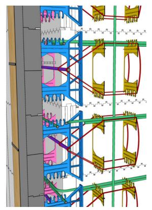
Figure 17 – Section view showing location of #5 (15M) bar and zip ties
