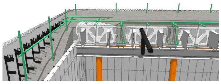
Figure 39 – Section view of Amdeck Pro
