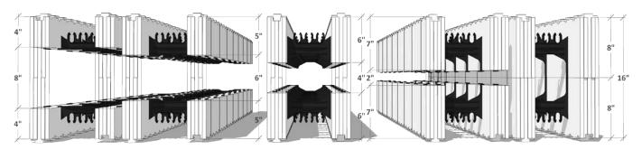
Figure 49 - Site fabricated height adjusters with the web intact provide additional strength
