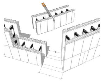
Figure 50 – Use hand saw or hot knife (not shown) to cut blocks to size
