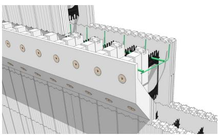
Figure 30 – Once the foam extension is attached, place reinforcing into the cavity
