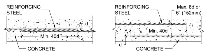
Figure 2 – Contact lap splices (left) and non-contact lap splices (right)
