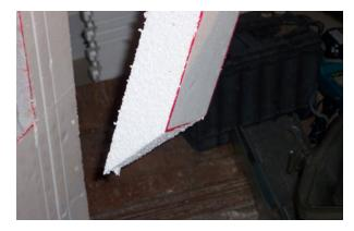
Figure 44 – Making the end cuttings flare out
