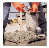
Figure 5 – Concrete mix with high slump
