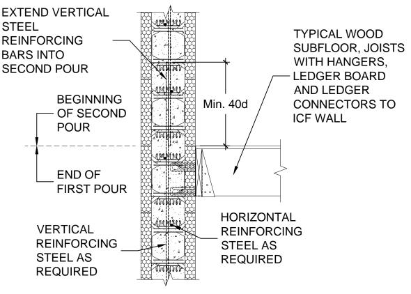
Figure 3 – Vertical lap splice
