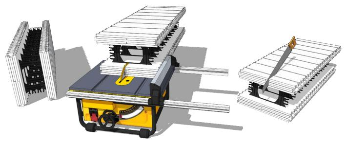
Figure 48 - Site fabricated height adjusters can be manually cut using a hand saw or a table saw
