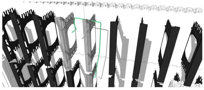
Figure 45 - Place the bottom of the hook under the top portion of the lower block's web
