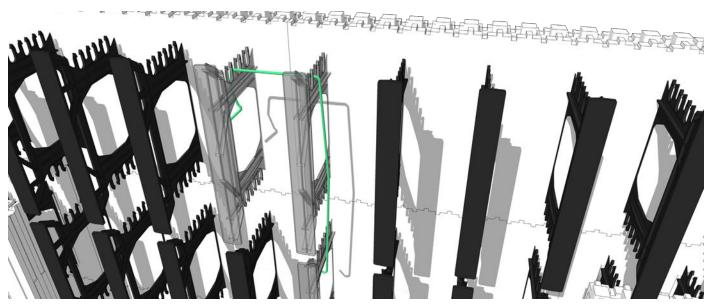
Figure 46 - Bring the top portion of the hook up and over the top of the two webs and snap it in place (pull the lip up to unhook it)
