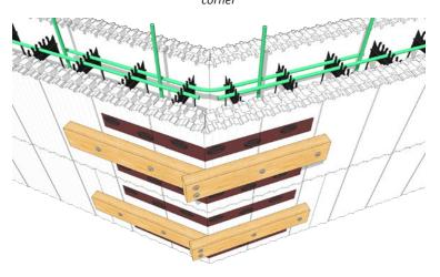
Figure 52 – For shorter walls (<4' (1.2m)), use horizontal bracing
