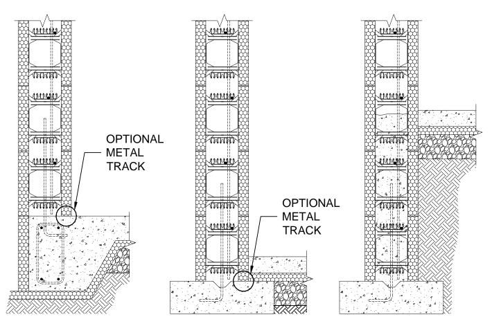
Figure 1 – Typical ICF footing types
