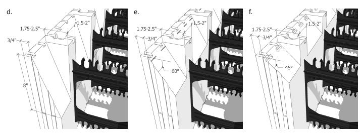
Figure 54 – Half block height cut-out (d), 60° cut-out (e), 45 ° cut-out (f)
