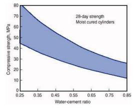
Figure 2 – Relationship between W/C ratio and concrete strength
