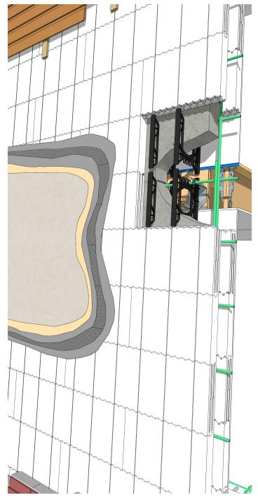
Figure 1 – Typical stucco application over ICF
