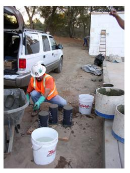
Figure 12 – Taking random samples of concrete for compressive strength testing at 28 days
