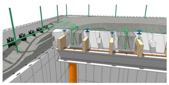
Figure 40 – Section view of Amdeck Eco
