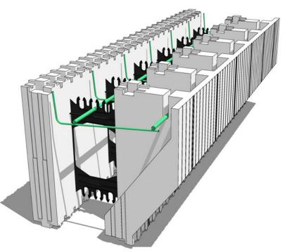
Figure 27 – Place the Reinforcer into the form. No additional tying or securement is needed.
