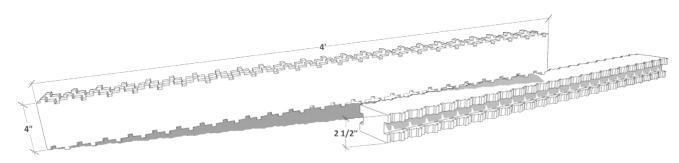
Figure 47 - 4" (102mm) double side factory fabricated height adjuster (available for both R22 and R30)
