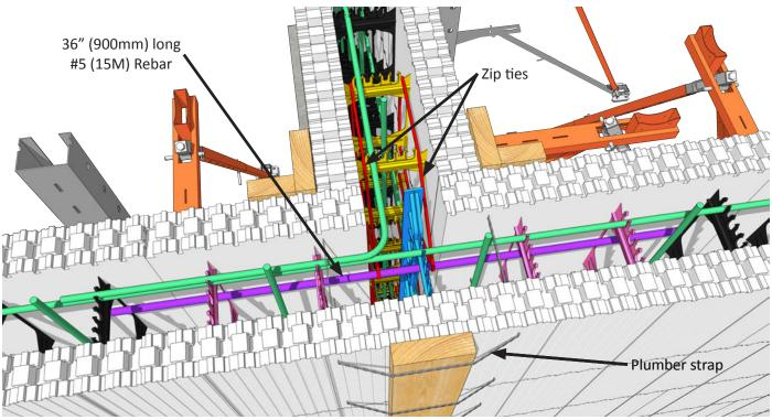
Figure 18 – Typical site constructed T-wall connection using straight blocks
