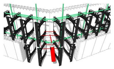
Figure 51 – Use spray foam and zip ties to help secure site constructed 45° corner
