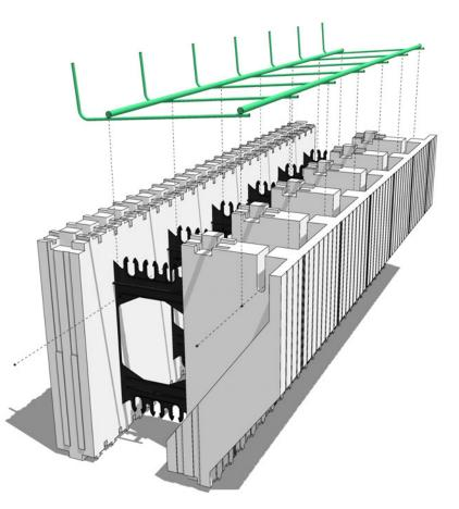
Figure 26 – Align Amvic<sup>™</sup> Brick Ledge Reinforcer with notches in the foam and the clips on the webs.
