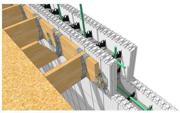
Figure 53 – Attaching floor joists to the ledger board with the Simpson-Tie™ (ICFVL-W with dimensional lumber shown)
