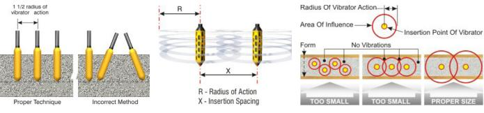
Figure 14 – Vibrator head placement
