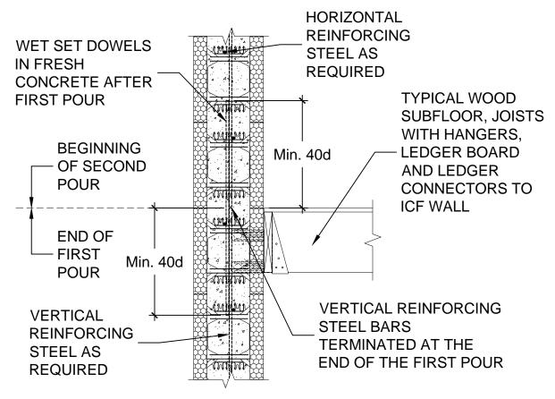
Figure 4 – Vertical lap splice using a dowel
