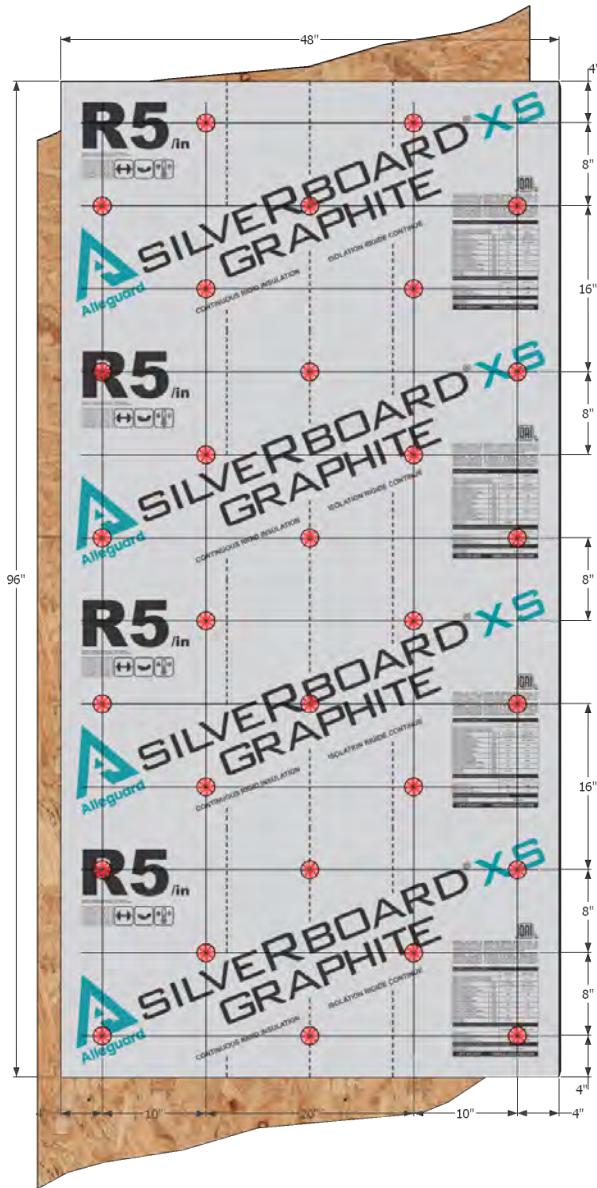
Figure 5 – Vertical nailing Pattern A (30 assembled fasteners)
