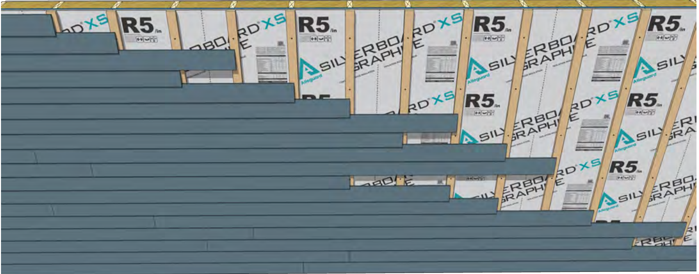
Figure 21 – Horizontal wood/composite siding with wood strapping on 2-1/4 (57mm) SilverBoard Graphite XS
