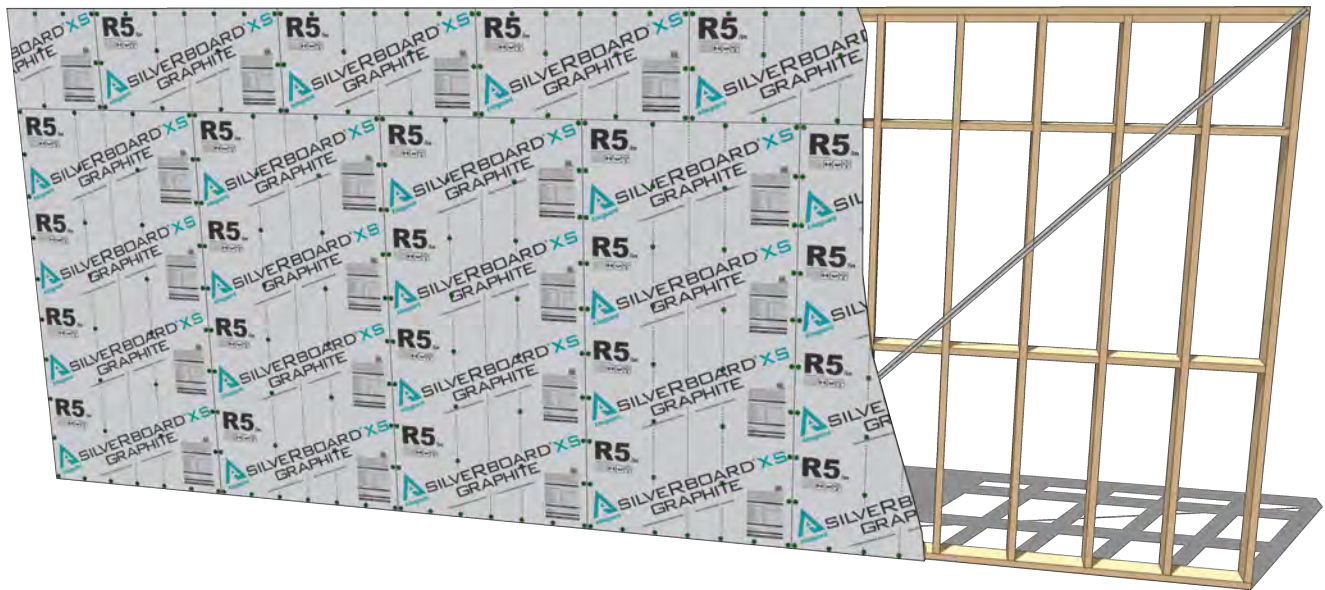
Figure 3 – Vertical SilverBoard installation over open stud wall assembly
