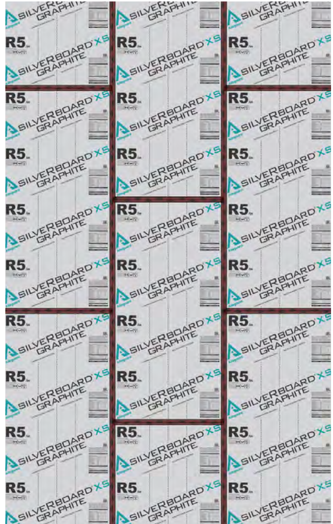
Figure 17 – Taping pattern for vertical board orientation
