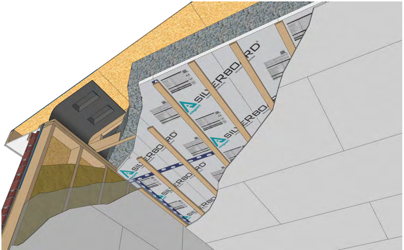
Figure 1 – 2" (51mm) high density SilveRboard installed with furring strips to underside of wood trusses
